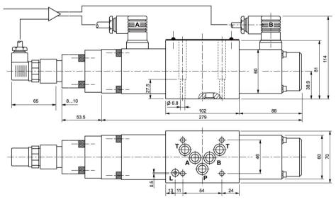
Dimensions of mounting hole configuration NG 10 ISO 4401 (Additional port L)
